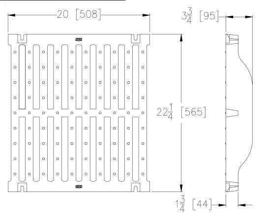
**ENGINEERING SPECIFICATION:** The Zurn -GDF, Galvanized Ductile Iron Slotted Grate, is 22-1/4" wide x 20" long, weighing 73.4 lbs per linear foot. The grate has an open area of 94.1 square inches per linear foot, DIN Rating of Class F, ANSI Rating of Special-Duty, H-20 Load Rated and FAA Load Rated.
